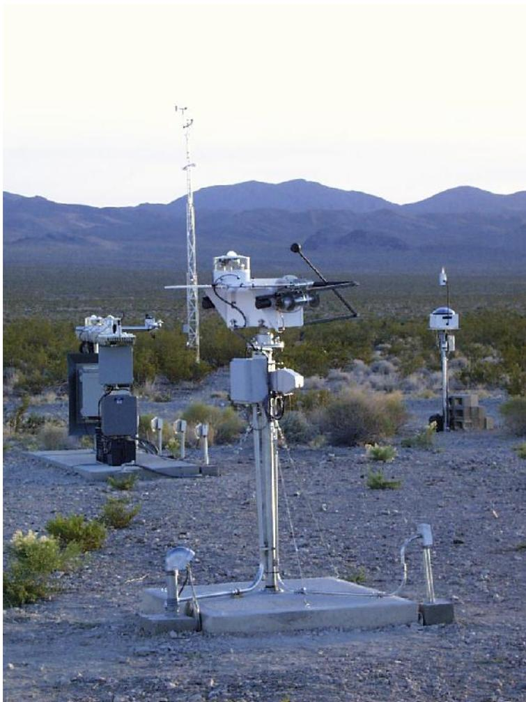
**Figure 6** – Example of a SURFRAD station, here showing the Desert Rock (Nevada) station. Clockwise from left center: Radiometer platform, met tower, total sky imager, and solar tracker. From <http://www.esrl.noaa.gov/gmd/grad/surfrad/>.
